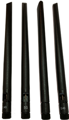
Internal WiFi Antennas (x4)
