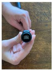
15. Push the insert into the Weatherproof plug and secure the cap back on the Weatherproof plug. The insert has a groove that is required to line up on the inside on the plug.
