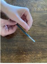
7. Untwist and straighten the wires inside of the cable.
