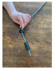
4. Strip the Starlink cable sheath back 25 mm from the end.
