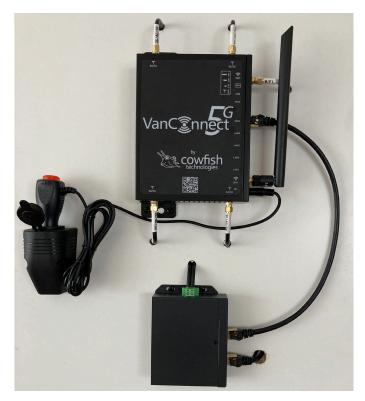
In order to supply input power to the 12V Dishy Power Supply, a minimum of 14 AWG electrical wire is required. This cable is to be connected to the 12V power source and correctly fused. Installation by a certified auto electrician is advised. The 12V Dishy Power Supply comes with a pluggable terminal block for easy wiring. Connect the 12V positive wire to the terminal labelled + and the 12V negative wire to the terminal labelled - When correctly installed the Power In LED will turn on.
